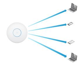
MU-MIMO with 1x1 clients: The UniFi HD AP communicates with four 1x1 clients at a time.
