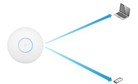
MU-MIMO with 3x3 and 1x1 clients: The UniFi HD AP communicates with one 3x3 client and one 1x1 client at a time.
